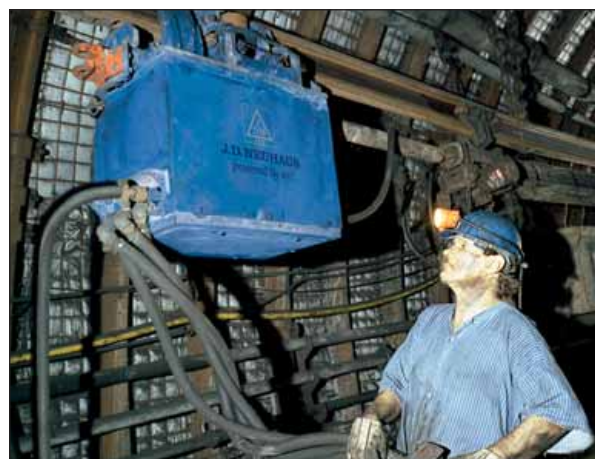
JDN Shunting Trolley SK 125 working underground.
